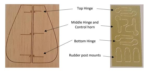
Be careful as when the hinge components are cut from the CNC'd epoxy board they are small and can easily be lost.
