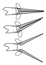
2. Method used on the Midge: By using CAD and a CNC router machine, I have produced some hinges on epoxy board that allow for symmetrical movement. These use a central hinge system that pivots around a single piece of thin piano wire inserted through all three hinges from the bottom. The hinges consist of left
