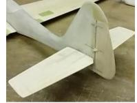
Once you are happy with the functional rudder installation, then remove the rudder halves by pulling the centre hinge pin out. The rudder assembly is now ready for covering. I used 80 gram cloth and epoxy resin for this, but you could use other covering material.
