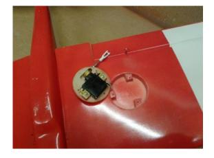
6. Cover servo recess with suitable cover. Either epoxy sheet or plastic card or moulded fairing. The moulded fairing provided should be reinforced with a 1.5mm plywood disc epoxied into place.
