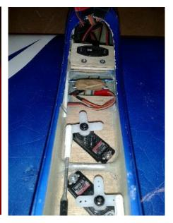
10. The Battery and receiver can be installed directly in front of the wing inside the fuselage, but installation is easier and more practical by fastening them onto a ply or plastic card plate that slides into the front of the fuselage in front of the main wing joiner. This will keep the installation neat and tidy and help with the removal of the gear if necessary. A small plywood plate can be screwed into place over the main wing joiner hold the radio plate secure if necessary.
